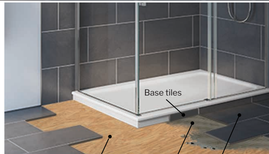
Plywood subfloor Tiles adhesive Floor tiles
